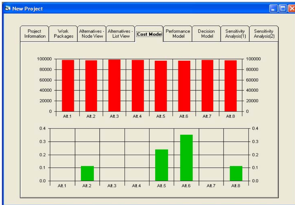
Figure 7-11. Cost Model Shows the Analysis Results (Weights) of Cost for Each Supply Chain Alternative. Red Bars Show the True Cost of Each Supply Chain Alternative and Green Bars Show the Cost Weight for Each Supply Chain Configuration.
